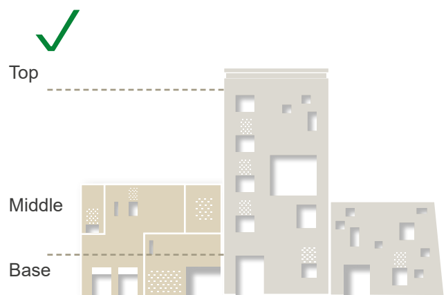
FIG. 31 Facades loosely defined in three parts with articulation of openings
