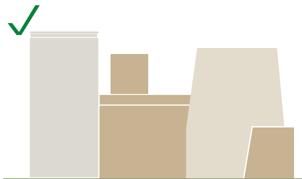
FIG. 24 Masses broken into primarily vertical volumes with balance of horizontal volumes to achieve human scale and variation in skyline
