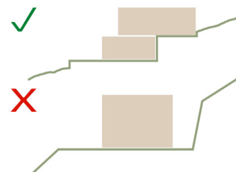
FIG. 23 Built form respecting the natural terrain to be encouraged; large flattening of sites should not be permitted
