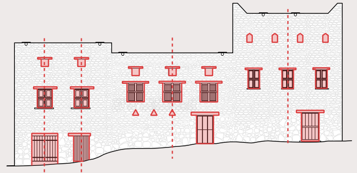
FIG. 13 Variation and asymmetry in openings Facades are punctuated by a range of opening sizes and shapes - positioned asymmetrically.
