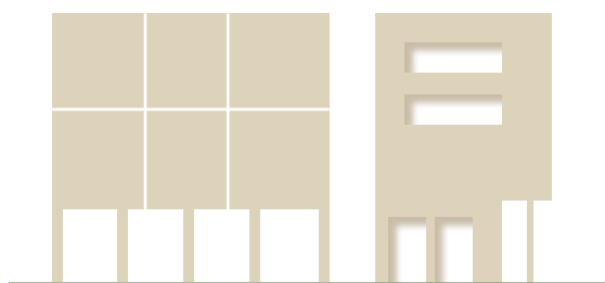
FIG. 31 Very large openings at base, thin columns, blank, recessed ground floors, non-integral facades, lack of respect to privacy needs, should be avoided
